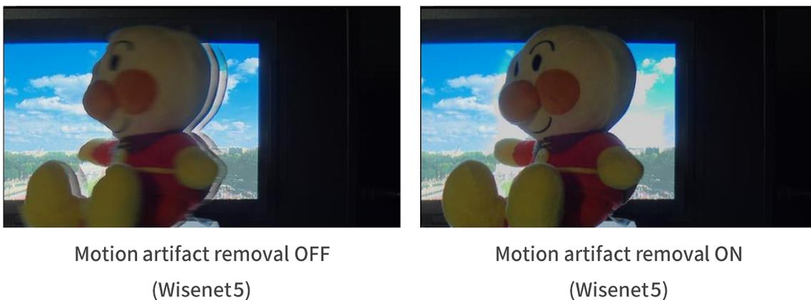
Figure 7. Effect of Motion Artifact Removal in an X series (Wisenet 5) product
