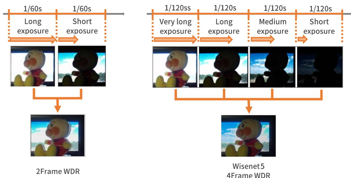
Figure 5. Comparison of the existing 2 fps WDR and 4 fps WDR applied to X series
