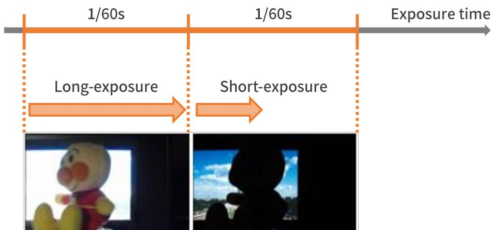
Figure 2. Process of obtaining long-exposure and short-exposure images
