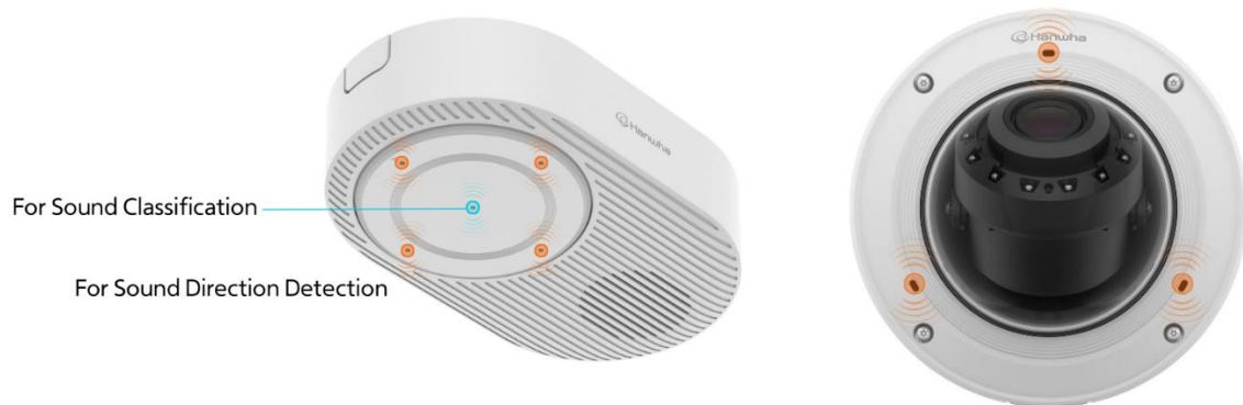
Figure 3: Microphone Locations on Audio Beacon SPS-A100M (Left) and Wisenet 9 Cameras
