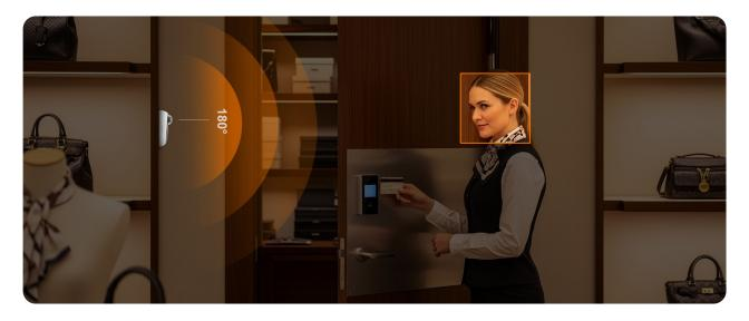
This camera offers an eye-level perspective, capturing details that might be missed with traditional surveillance positions. Featuring built-in AI analytics and IR, its panoramic lens provides nearly a 180° field of view while recording high-quality 5MP resolution video for better object identification.
