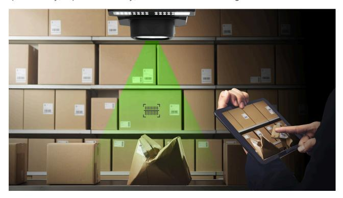
With an integrated logistics system (WMS) and CCTV system (NVR), the Hanwha Vision VLTS enables operators to easily track a package and access video playback by simply scanning the invoice barcode.
