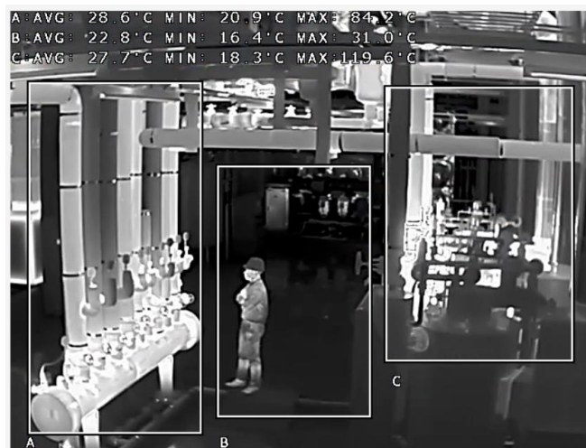
[Figure 17. An example of average, maximum and minimum temperatures depending on areas of ROI]
