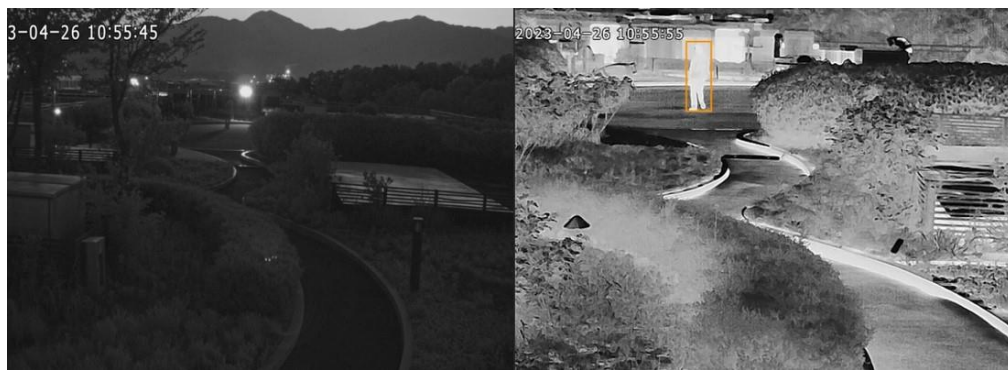
[Figure 15. Visibility difference between visible camera (left) and thermal imaging camera (right) in a night environment]
