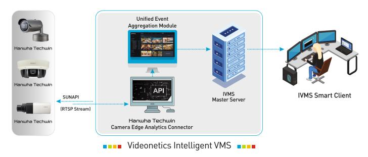
Intelligent VMS 3.0 uses PUSH mechanism to receive event metadata from Hanwha Techwin cameras. Videonetics IVMS has a software 'connector' to link up with any compliant IP cameras event metadata stream through RTSP (i.e., event information in XML format) from the cameras.
