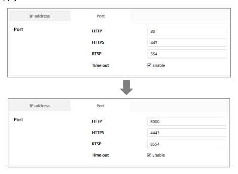
• When port number is reassigned, it may cause communication problem if there is a connected recording device or VMS. If not resolved, return to the default port, please.
