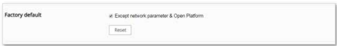
If you physically press the reset button on the camera, all settings, including network settings and open platform information, will be initialized to the factory default.
