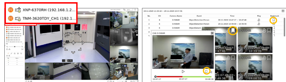
Live monitoring and PTZ control
