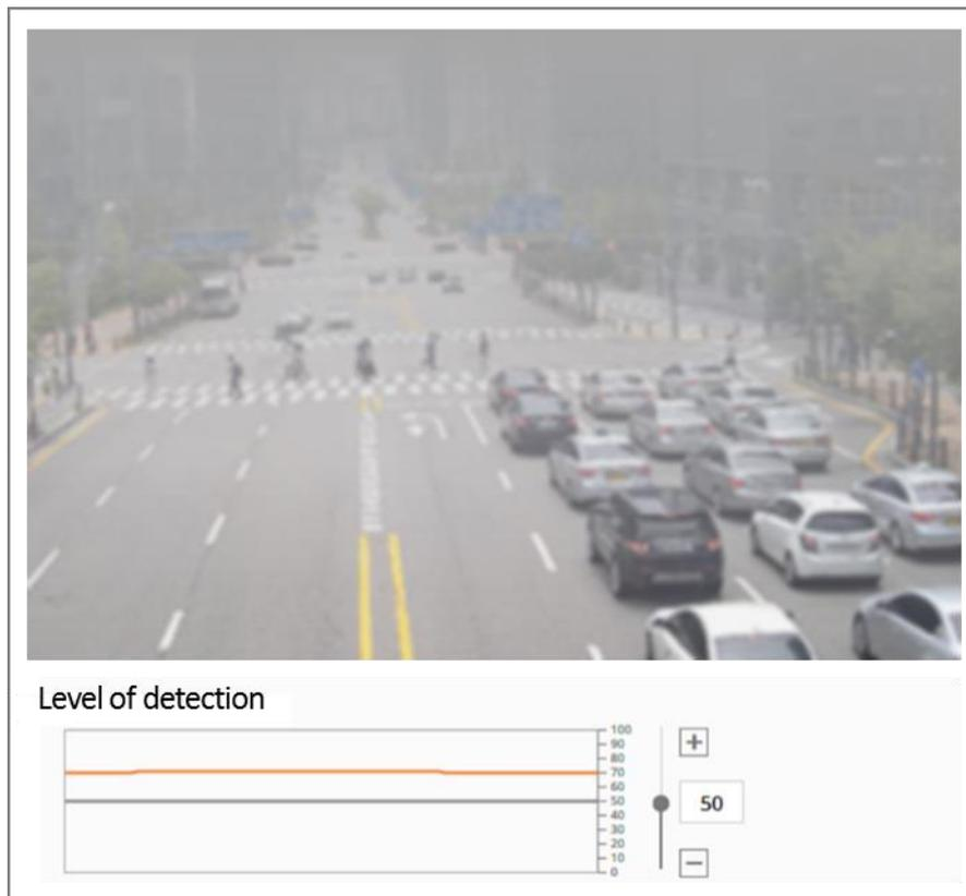
Figure 2. Example of Foggy Image and Level Graph
