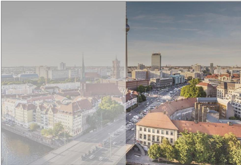
When the visible distance is shorter due to fog or dust in the air surrounding the camera, it reduces color and edge information, resulting in a significantly lower recognition rate in image processing. In areas that require full-time outside monitoring, such as airports and ports, a function for removing fog, which counts as noise, is crucial to improving the recognition rate.
