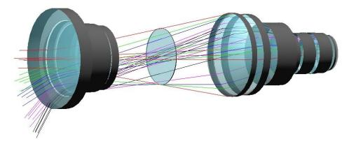
Image 1. E.g. Image of lens design for correction of various incident angles of light
